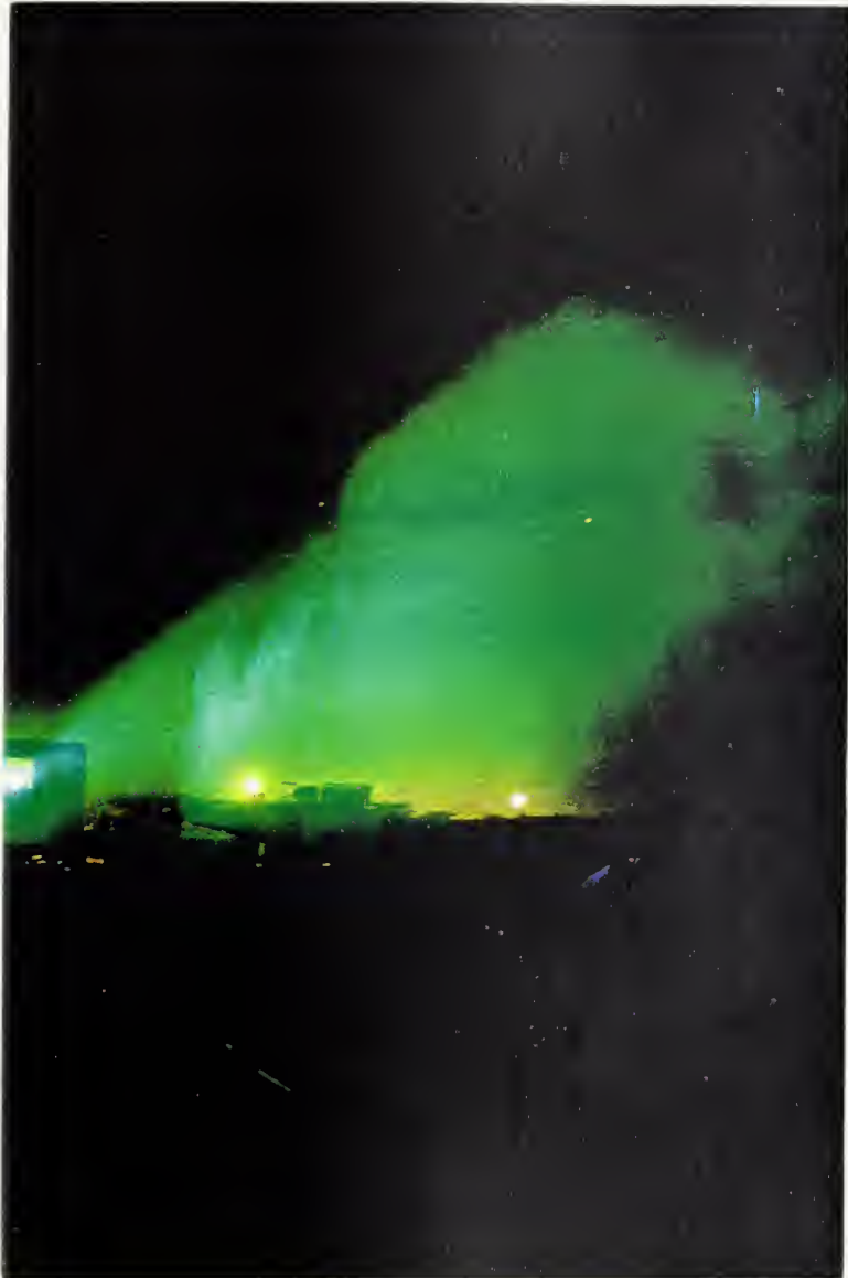
Figure 2.7 With the camera located near the end of the pier at Moss Landing, the laser fan is visible with stronger forward scatter from developing plumes.
