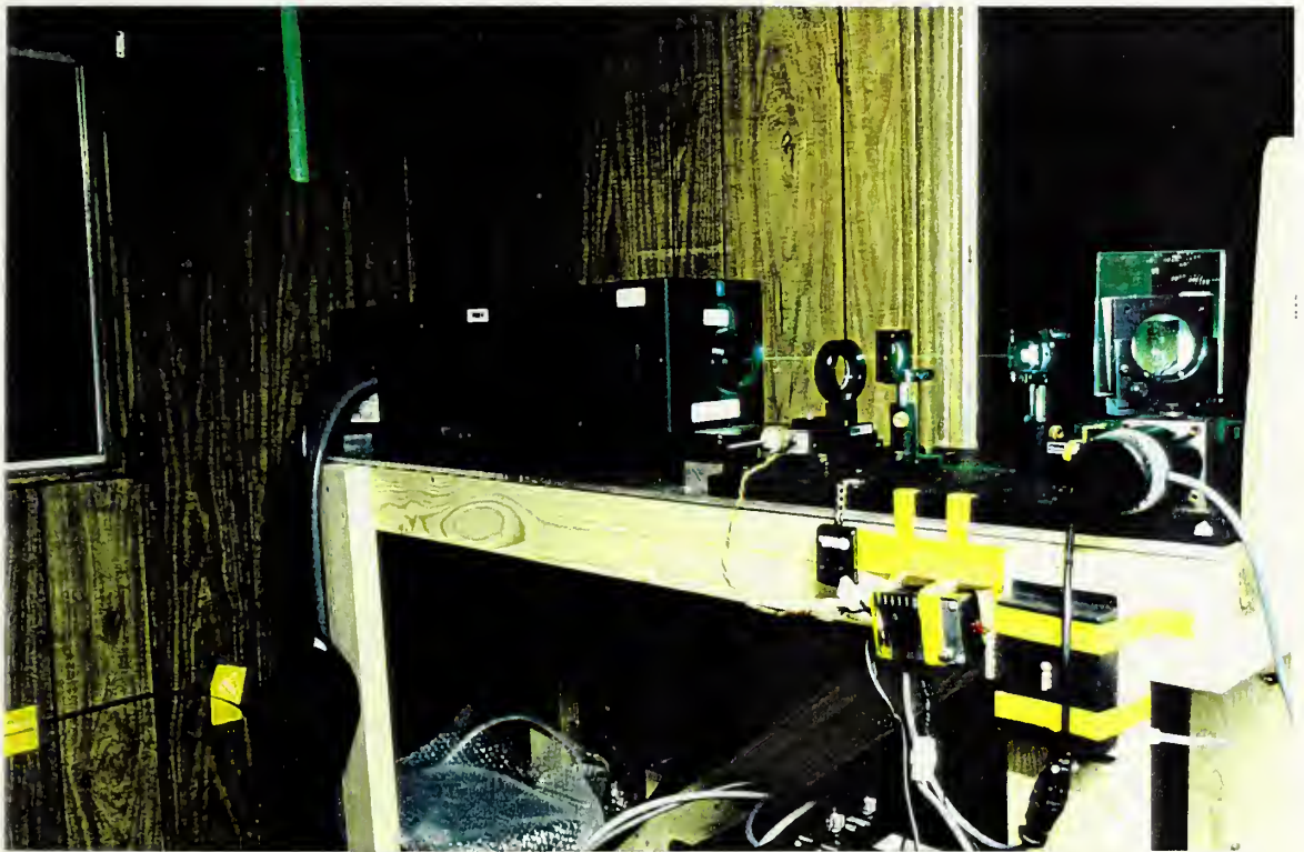
Figure 2.4 Penn State's Laser Scattering 514.5 nm Argon-ion (green) laser configuration from emitter through negative cylindrical lens, polarizer and reflecting mirror.
